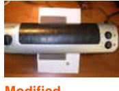
Modified laminator for PCB Toner transfer by hobby16
