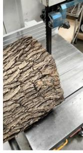
Cutting with a cradle or jig is allowed (makes sure you do not cut any screws used to hold the 2x4 to the plywood). The cradle/jig provide support for the log and will prevent spinning/rolling. Note: DMS does not provide cradles or jigs – you need to make your own. The jig is based on a design found in Wood Magazine https://www.woodmagazine.com/woodworking-plans/jigs/resawing-bandsaw-jig-and-
