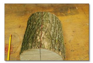
Figure 13: Connect the ends of the plumb line to locate the centerline of the blank as shown. Mark the approximate center of the line so you will know where the circle will be cut.
