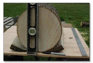
Figure 3: The initial plumb line drawn in will establish a reference line on both sides of the log section and will allow you to lay out two parallel blanks on either side of the pith.
