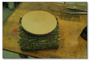
*Figure 14: The circle screwed to the blank is easy to follow with the band saw. This method is much easier and more accurate than trying to draw a circle with a compass.*
