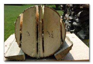
Figure 8: Don't cut all the way through the log when making the initial cuts. The log will be more stable and safer done this way. Once all the cuts are made, you can go back and finish the cuts starting with the two outside cuts.
