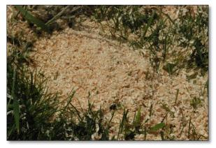
Figure 6: The shavings shown are the kind normally produced when crosscutting with the chainsaw. They are easily discharged from the saw and usually don't present a problem.
