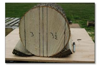
Figure 4: You do not want the pith to be present in either blank so the first lines drawn are to eliminate it. You will note that I drew two lines adjacent to the initial line, 1-1/2" apart I then laid out the two blanks with the level, making sure that the lines were plumb. The other end is the mirror image of this end.
