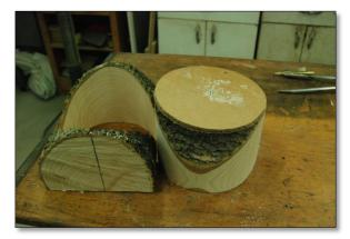
Figure 15 shows the final result after cutting out the circle on the band saw. I have a number of circles of different diameters that I use for natural edge bowls. The templates will last for quite a while if you are careful when cutting and just rub the outside of the pattern with the blade.
