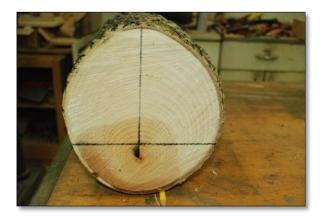
Figure 12: Draw a plumb line through the pith and then draw a perpendicular line that intersects it as shown. This is done on both ends and will allow you to locate a centerline that corresponds with the centerline of the blank.
