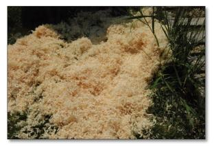
*Figure 7: The ripping cut produces long, wispy shavings shown. Be careful that they don't clog the discharge chute of your saw.*
