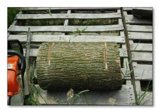
Figure 2 shows the log laid out, ready to be cut to length. I cut the section out in the middle of the log in order to eliminate any cracking that was present on the ends. You will have to keep reducing the length until all the cracks are gone, even if it means working with a smaller blank. There is no point in trying to turn cracked wood! Try to get as square a cut as possible when cutting to length.
