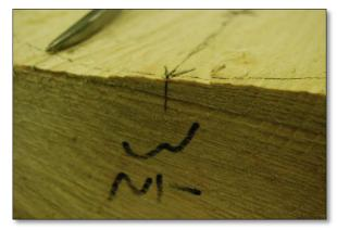
Figure 9: Locate the approximate pith center on both ends of the blank and draw a line through it as shown. This will help you to center the blank and the grain pattern in the resulting bowl will look more balanced.
