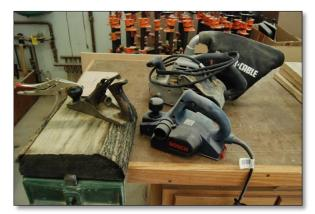
Photo 4 shows the tools that could be used to flatten the blank enough to cut successfully with the bandsaw.
