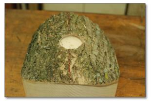
*Figure 17: Drilling a large hole through the bark and inner layer provides a stable rest for the spur center.*
