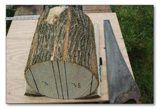
Figure 5: The lines on the top of the log will show you where to cut with the chainsaw. They are much easier to see when cutting than if I had drawn them with a marker. They don't have to be cut very deep, just deep enough to score the bark.
