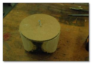
Figure 16: Locating the bottom is easy using the method shown. Most natural edge bowls start mounted between centers, and knowing where the center of both ends is located saves time and is more accurate.
