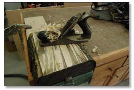
Photo 5 shows what just a few strokes with the hand plane will do to the surface of the blank. The plane will cut the wet wood fairly quickly and will make short work of smoothing out a blank that wasn't too rough.
