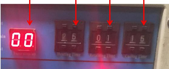
When the foot pedal is clicked, the Cycle Timer will track each cycle's timer (Heat/Hold/Cool) in sequence
